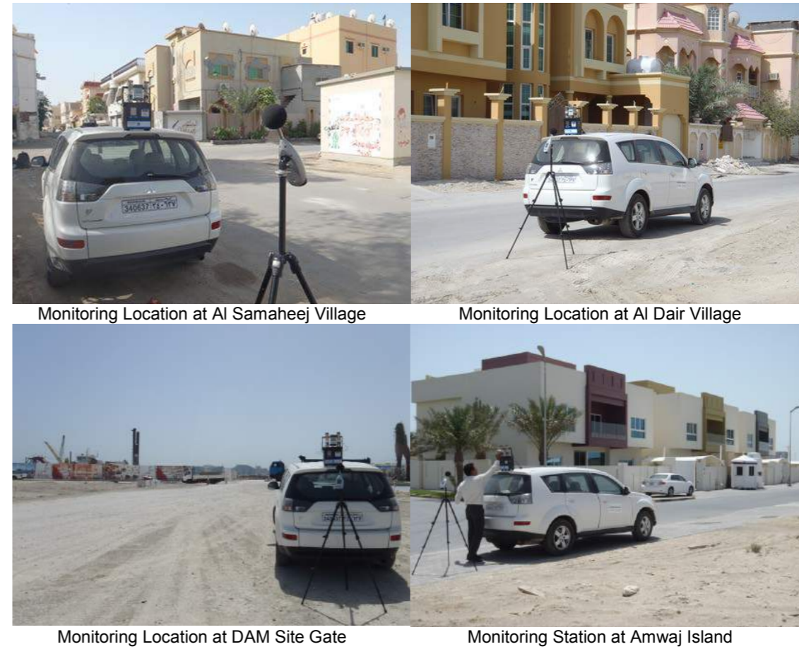
Figure 2.7: Photographs of Air and Noise Quality Monitoring Stations
