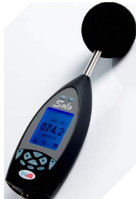
Figure 2.8: Noise Monitoring Instrument and its Specifications
